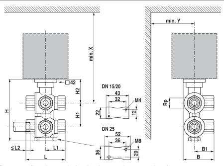
The actuator dimensions can be found on the respective actuator data sheet.
