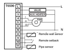
Application 6: Two pipe heating or cooling with Auxiliary electric heater wiring diagram (T6590B1000 only)
