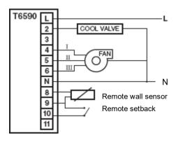
Application 1: Two Pipes, Cooling-Only wiring diagram
