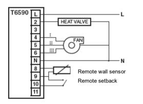
Application 0: Two Pipes, Heating-Only wiring Diagram
