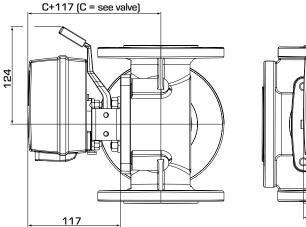
Installation dimensions for Actuator Series 90
