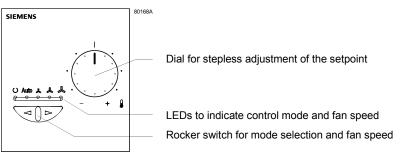
Rocker switch for selection of mode and fan speeds
